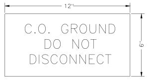
Self-Adhesive Nameplate 1/8" Phenolic Laminate Red Face with White Lettering
